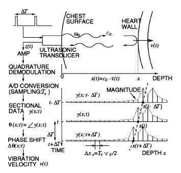
Fig. 1. Schematic representation of the transcutaneous measurement of a heart wall vibration, v(t), from the chest wall using pulsive ultrasound based on the standard procedure when the object position does not vary so much.
