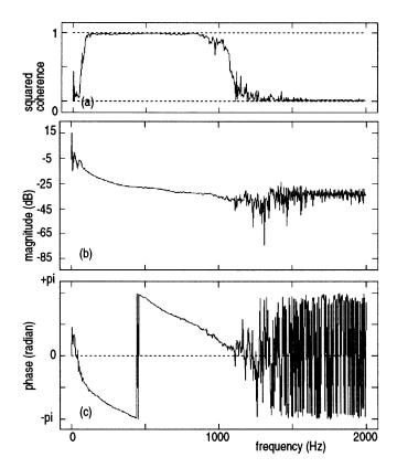
Fig. 10. (a) The squared magnitude of coherence function  $|\gamma_{in \leftrightarrow us}(f)|^2$  between  $V_{in}(t)$  and  $\hat{v}_{us}(t)$ , (b) the magnitude of the transfer function  $H_{in \rightarrow us}(f)$  from the input signal  $V_{in}(t)$  to  $\hat{v}_{us}(t)$  estimated by the proposed method in the frequency range up to near the Nyquist frequency  $1/\Delta T$ , and (c) the phase characteristics of the transfer function  $H_{in \rightarrow us}(f)$ .
