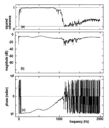
Fig. 11. (a) The squared magnitude of coherence function  $|\gamma_{laser \leftrightarrow us}(f)|^2$  between  $v_{laser}(t)$  and  $\hat{v}_{us}(t)$ , (b) the magnitude of the transfer function  $H_{laser \rightarrow us}(f)$  from  $v_{laser}(t)$  to  $\hat{v}_{us}(t)$  estimated by the proposed method, and (c) the phase characteristics of the transfer function  $H_{laser \rightarrow us}(f)$ .
