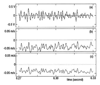
Fig. 9. To compare the high-frequency components of the waveforms in Fig. 8, (a)–(c) show the waveforms of the input voltage signal  $V_{in}(t)$  of the vibrator, the output signal  $v_{laser}(t)$  of a laser Doppler velocimeter, and the vibration velocity signal  $\hat{v}_{us}(t)$  estimated by the proposed method, respectively, during the period from 6.27 to 6.33 s in Fig. 8.
