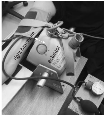
Fig. 2. Photograph of in vivo experiments in which right brachium artery is actuated with large scale actuator and velocity waves on heart wall are measured.
